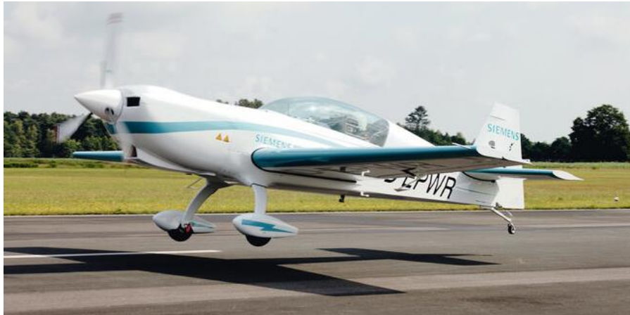
Fig. 1 Electric airplane Extra 330LE with Siemens electric engine
