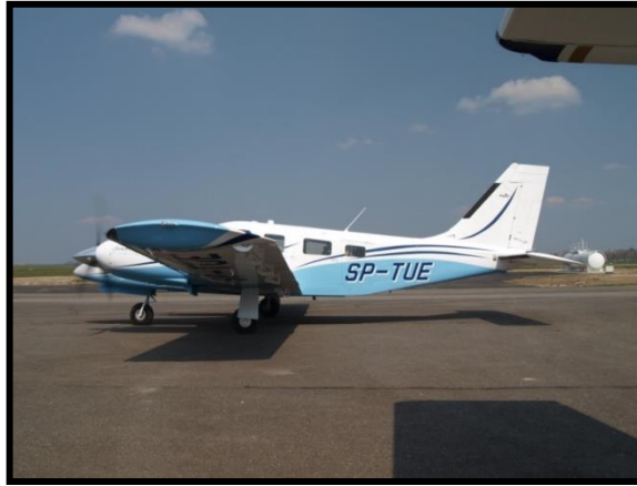
Figure 7 - Piper Seneca V (MTOW: 2155 kg, Never exceed speed: 378 km/h, 6 seats)
