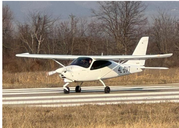
Figure 9 - Tecnam P2008JC (MTOW 650 kg, Max cruise speed 215 km/h)
