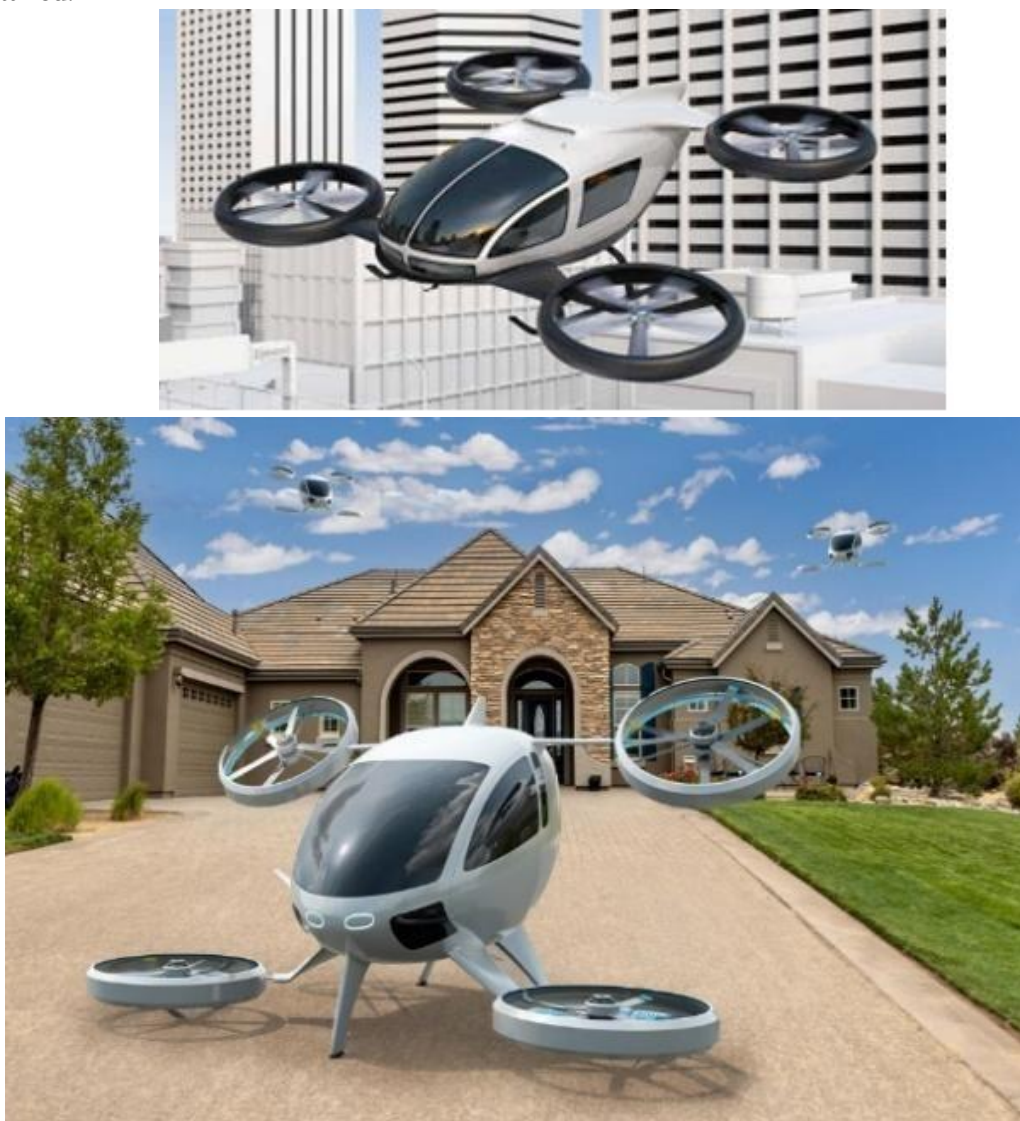
Fig. 3 Drones equipped with impeller-type ducted engines
