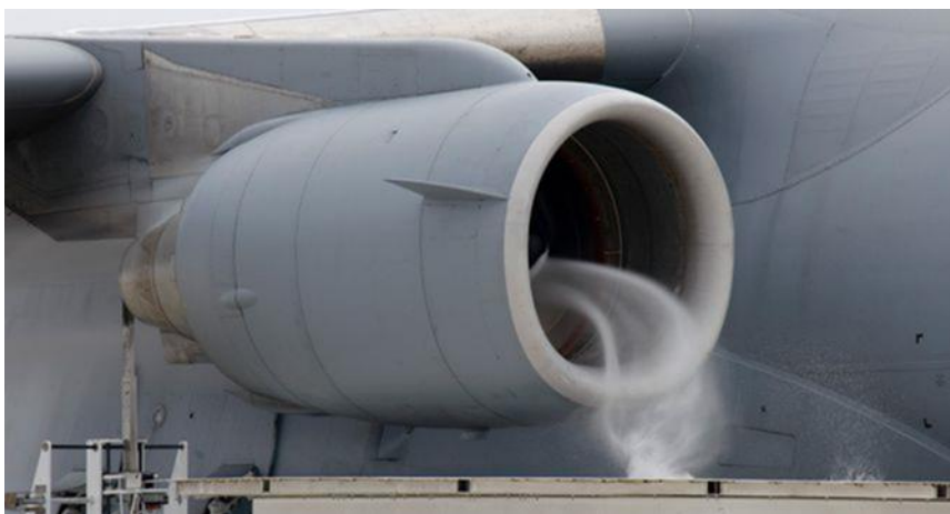
Fig. 1 Example of dust entrainment in the air intake of an aircraft gas-turbine engine
